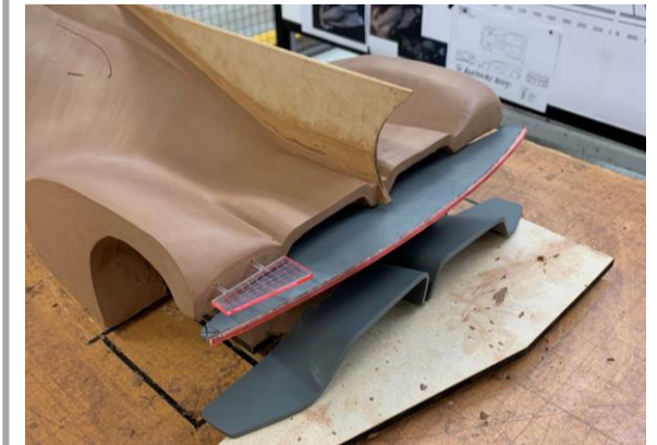
Adding final details to the roof scoop along with the DLO line to the cockpit and adding the painted rapid prototype parts.
