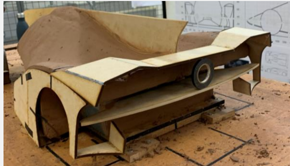
Forming the new design and early surfacing to it, and adding the fin
