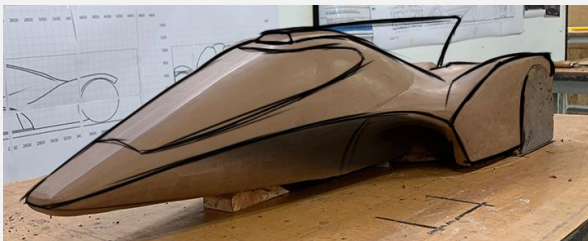
After feedback given the new design sketched over the model to improve the form. New design means that the driving position is moved to the centre
