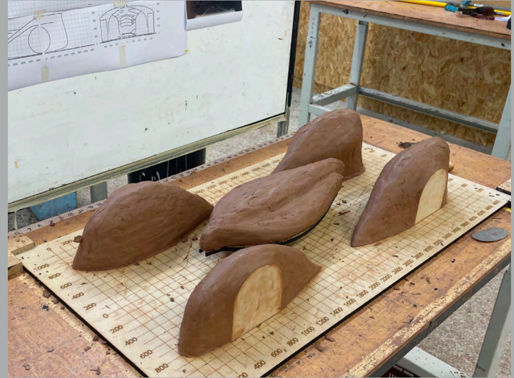
CLAY ROUGHLY BUILT UP TO MAX WIDTH
