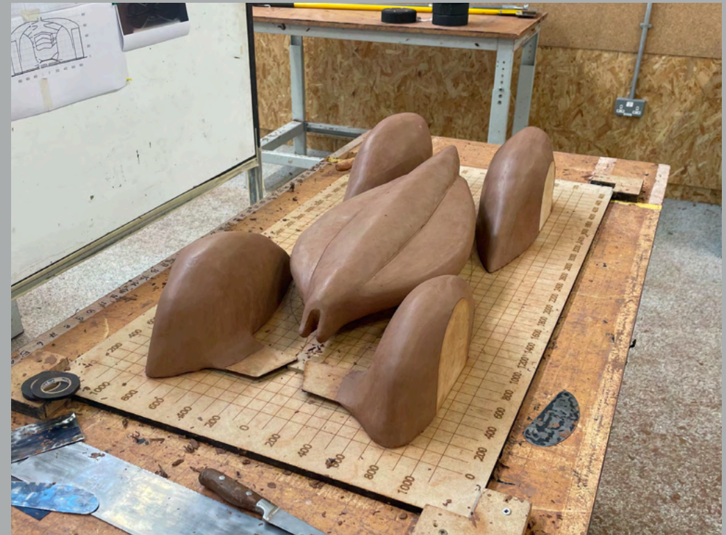
FULLY ROUGHING OUT MODEL AND FILING IN HOLOWS
