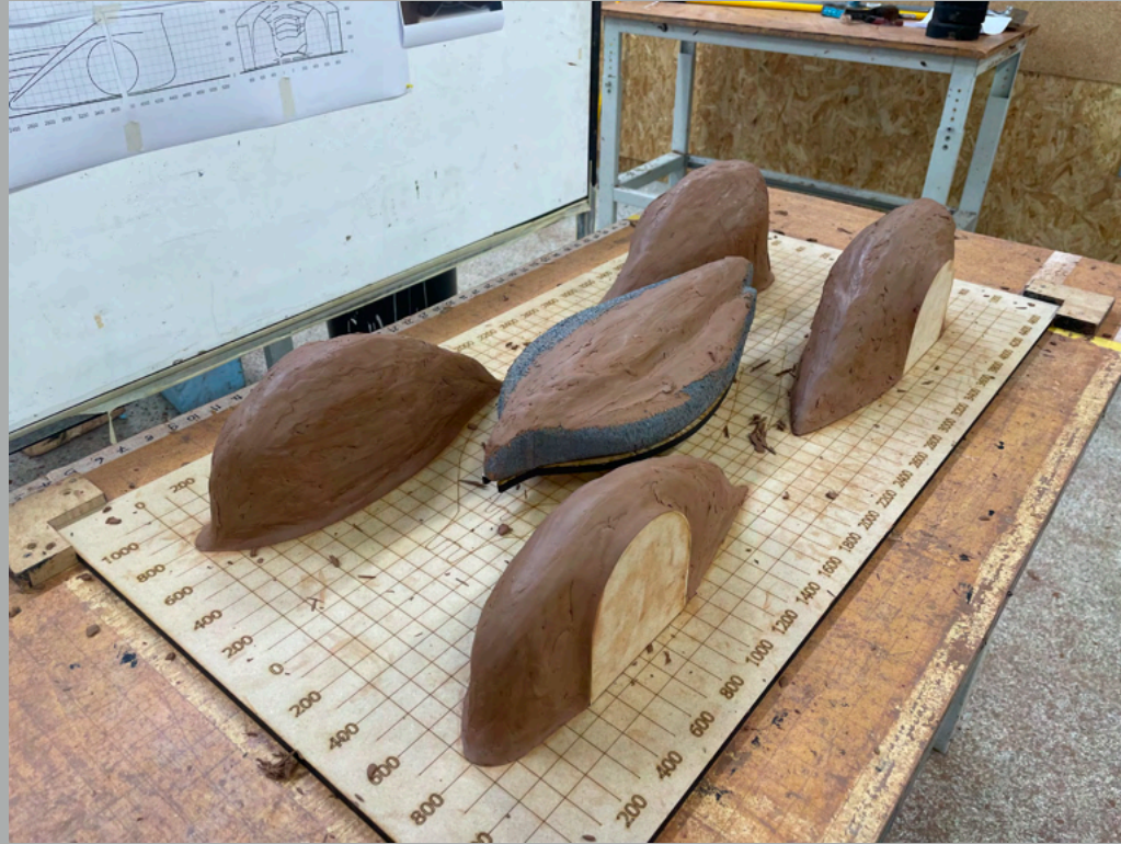
ADDING CLAY TO ARMATURE AND ADDING WHEELS
