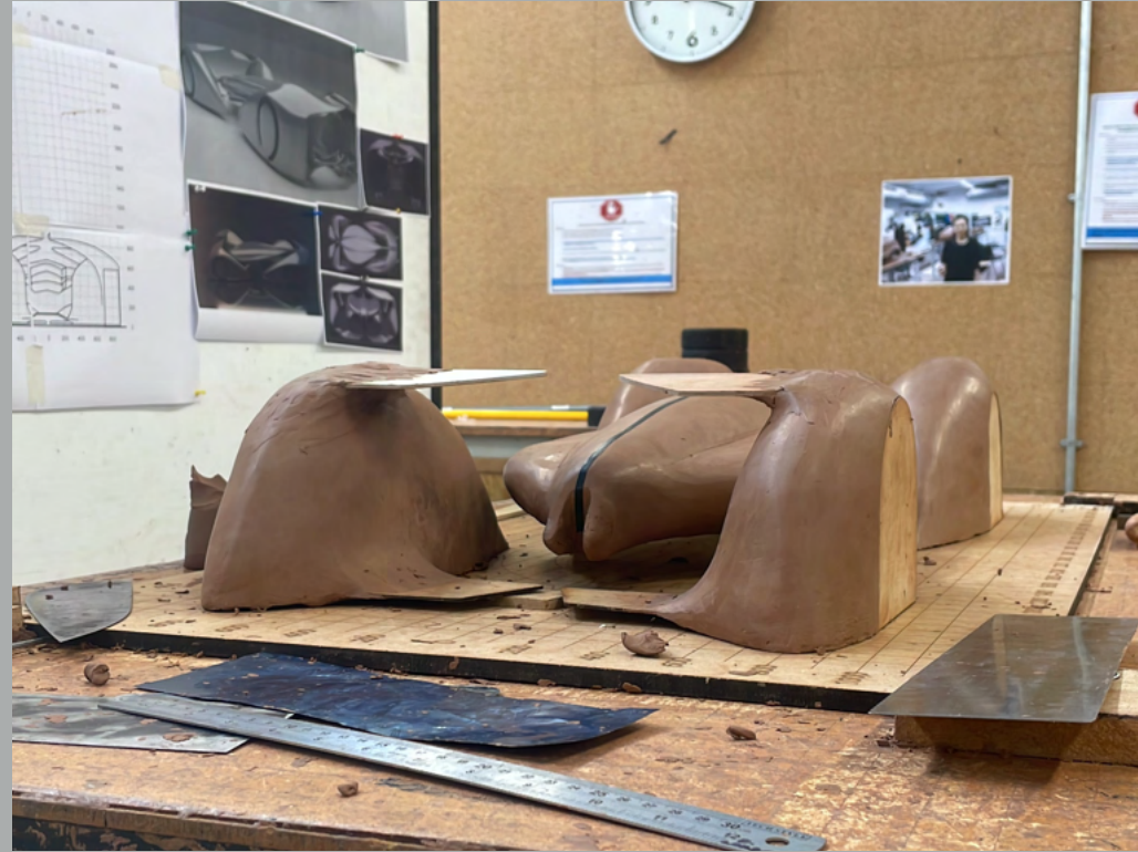
ADDING MORE AERO WINGS AND FURTHER FIXING SURFACE IMPERFECTIONS
