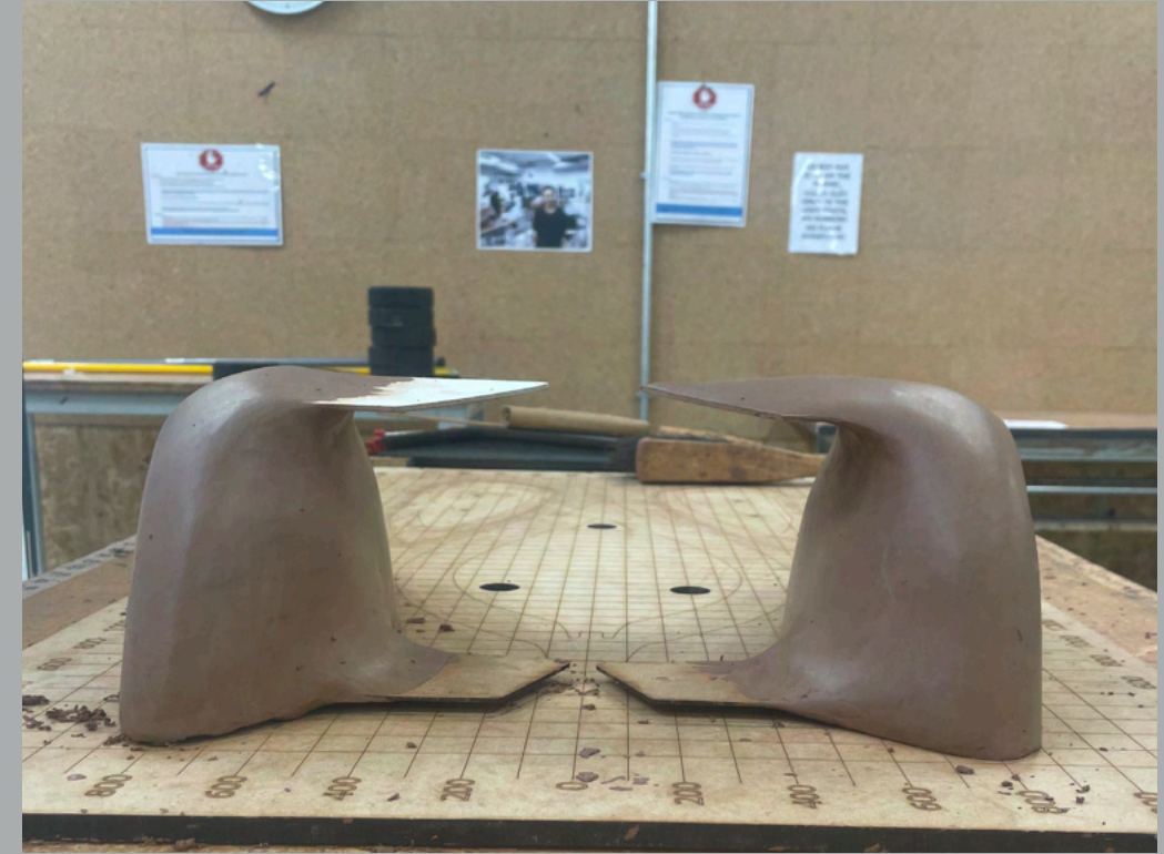
ADDING CLAY TO MAKE WINGS FLOW MORE SMOOTHLY INTO THE WHEEL ARCHES
