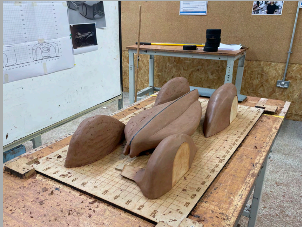
ROUGHING OUT ONE SIDE TO MAKE SURE PROPORTIONS ARE CORRECT AND ADDING AERO WINGS
