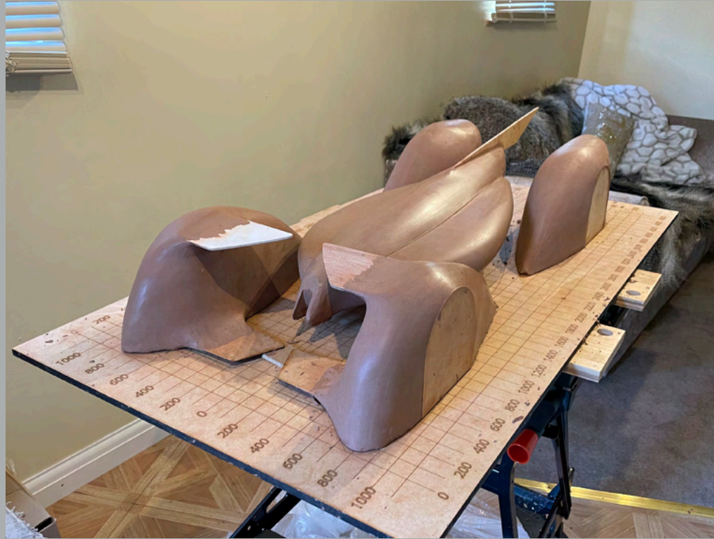
ADDED MAIN SPOILER AND FIXED FRONT VENTURI TUNNEL
