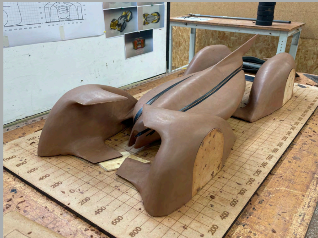
FURTHER REFINING SURFACE AND ADDING MORE REFINED LINES ON THE FUELTANK
